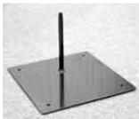
Black powder coated steel plate 1' x 1' x 3/16" thick with a 1/2" square 8" long steel post welded to the surface. This post goes up through the figure's shoe and heel, into a matching square steel tube inside the figure's leg. When used with the ETHAFOAM® Man the post goes into a sleeve that comes out the back of the calf. This heel plate can be used with the Flexible Foam Figure, Military Man Figure, and the ETHAFOAM® Man.
