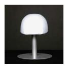
The Storage Hat Mount was designed for archivally appropriate storage of artifact headgear. It comes standard with a 6.75" diameter powder coated steel round base, and a 1" diameter anodized aluminum pole of various lengths, creating an overall height of 8", 11", or 15". The pole and base are available in silver or black. A 6.5" x 5" semi-sphere of ETHAFOAM® covered with a polyester stockinette fits atop the stand. Volume discounts available.
